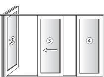
The second and subsequent panels slide up to the first panel and click into place.
