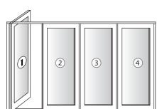
The first panel is fixed and can be on either side of the opening.
